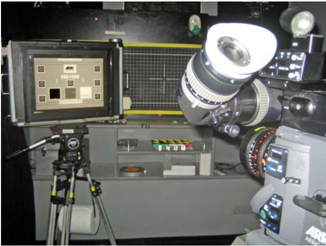
PI_Fig. 4: Setup for camera resolution test with transparent test pattern
