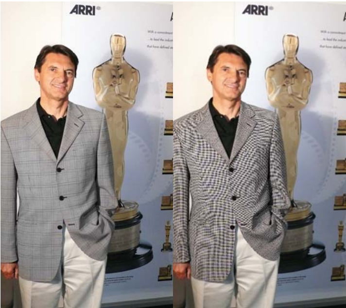
P2_Fig. 4: Digital still camera with 2 mio pixel Digital still camera with 1 mio pixel
