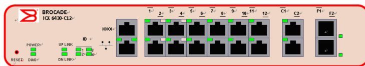
Figure 7. Front panel LEDs for the Brocade ICX 6430-C12.
