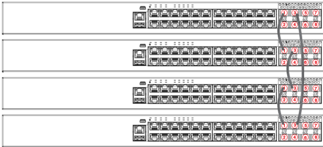
FIGURE 17 ICX 7250-24P Ring Stack
