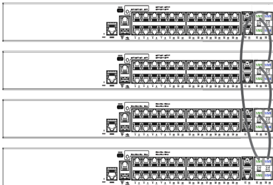
FIGURE 11 ICX 7150 24-port Stack Ring Topology
