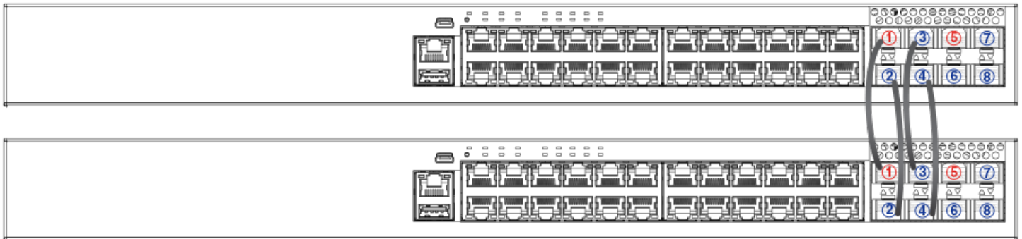
FIGURE 18 ICX 7250-24P Two-unit Stack with Linear-topology Trunk
